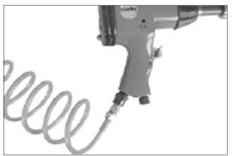
7. If using a mini oiler, place a sheet of paper next the exhaust port and hold the throttle open for approximately 30 seconds. The oil volume is correctly set when a light stain of oil can be seen on the paper. Excessive oil should be avoided.
